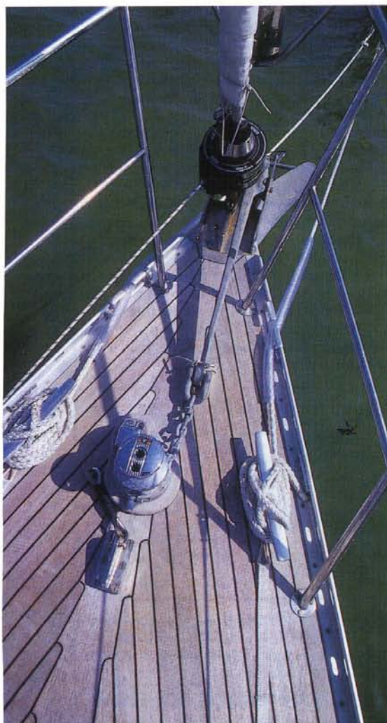
Below: The foredeck is uncluttered, easy to work on and sports twin bow rollers for double anchoring and cleats that wouldn't look out of place on a boat twice her size. An electric windlass draws the chain down through a hawse into a capacious locker below – one of the few arrangements that does feel a little old-fashioned. Those of us who regularly anchor at night would prefer not to have to run below every time the chain forms a pyramid, blocking the hawse. Having the windlass mounted below deck level and a self-draining chain locker with deck access is a boon for coastal cruising.
