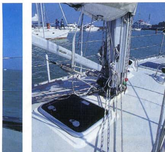
Above: On Little Dove , all lines are led back to the cockpit for ease of sail handling, but many have kept the reefing lines and halyards at the mast to clear the cockpit of too much string
