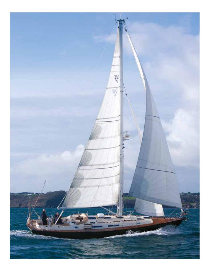
The Rustler 42 is immensely strong. Hull and deck mouldings are laid up by hand using quadraxial matting with isophalic resin. Bulkheads are fully glassed to the hull and deck. Together with substantial stringers and a lead encapsulated keel the result is a yacht with unrivalled strength and endurance.
